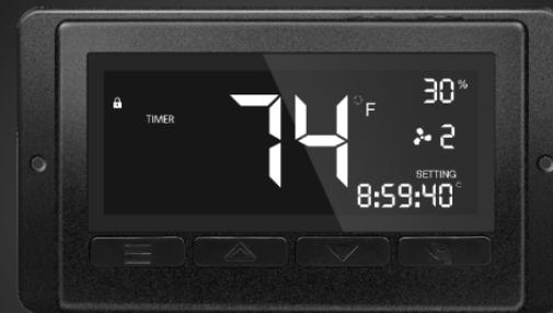
TIMER Mode, press the up or down button to set a time for the timer. The fans will run at the speed set in ON Mode until the timer's clock runs out, in which the fans will stop running. The clock will begin counting down if no buttons are pressed for 3 seconds. Leaving the timer mode while the countdown is running will pause the clock until you return to this mode.
