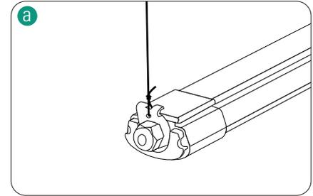
Attach the hanging rope to the hook on the light bar.
