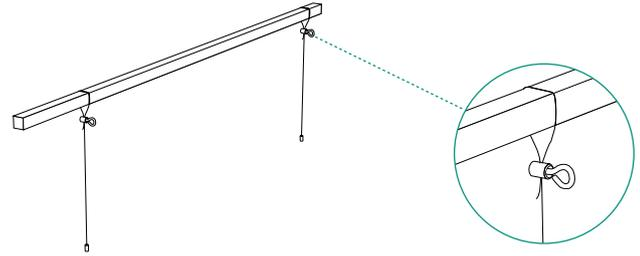
(4) Insert the clip and adjusted end through the loop of the cable .
