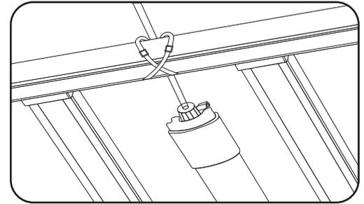
Use zip ties to secure the light strip to the main light frame
