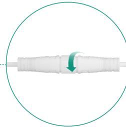
To disconnect the power cord, twist the two halves away from each other first then pull apart.
